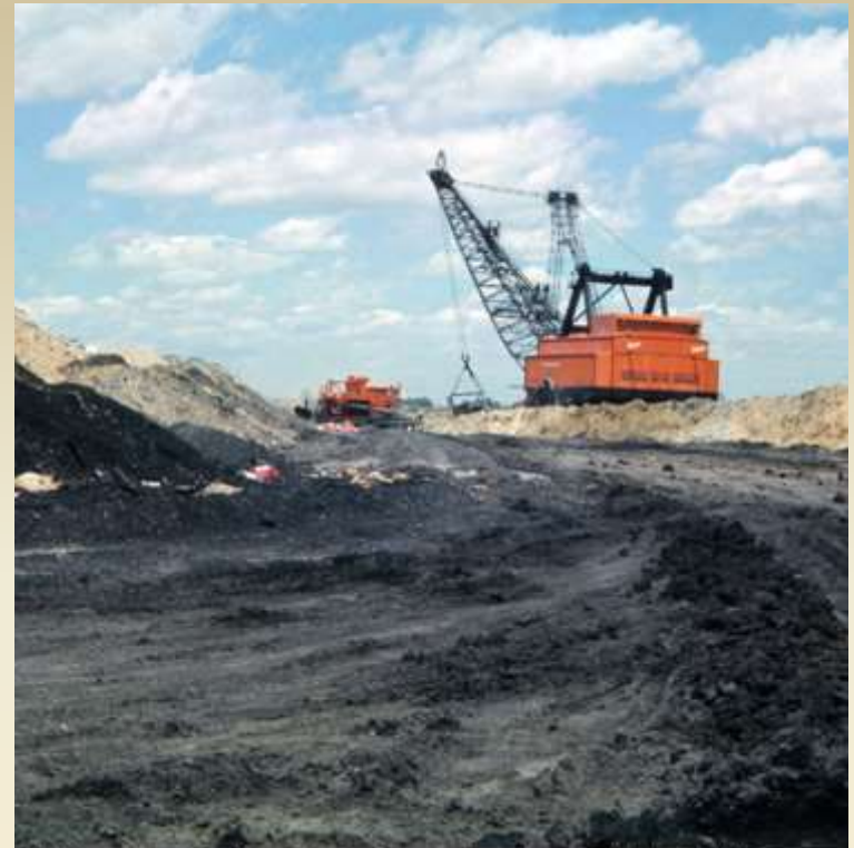
P&M Midway Mine. 110 cubic yard Memphis Queen dragline and horizontal drill, June 10, 1975.
